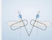
Automatic convergence and PD adjustment during near point test.
