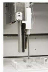
Sample/Reagent Probe with Liquid Level Detection
